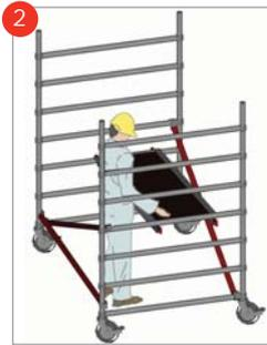
Attach diagonal braces in opposing directions from the 1<sup>st</sup> to the 4<sup>th</sup> rung. Attach platform to the 3<sup>rd</sup> rung (ensure trapdoor opens outwards). Check the base with a spirit level in both vertical and horizontal directions and adjust the legs if necessary.
