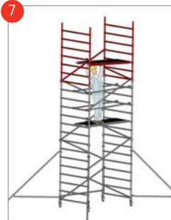
Fit additional standard frames and lock. Clip 4 diagonal braces from rung 12 to 18 in a zig zag pattern (opposing direction). Also move the trapdoor platform from the 3<sup>rd</sup> rung to the 17<sup>th</sup> rung.
