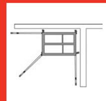
Lightly tighten the upper clamps above the sixth rung on each corner post. Position the lower clamp above the bottom rung. Ensure the lower arm is as horizontal as possible. Position the stabilisers so that the footpads are approximately equidistant from each other, as seen here. Telescopically adjust the leg and reposition the clamps as required to make firm contact with the ground. Ensure the clips with locking pin are in place. When in the correct position, tighten the clamps firmly.
