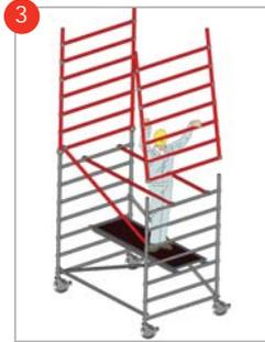
Fit guardrails (horizontal braces) to the 6<sup>th</sup> rung either side of the platform. Insert 2 standard frames to the lower frames, and insert locking pins.
