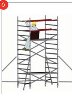
Using the 3T method, clip 4 horizontal braces on the 12<sup>th</sup> and 14<sup>th</sup> rungs on both sides of the platform
