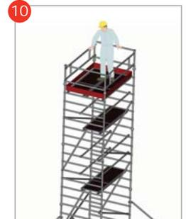
Fit 1 trapdoor platform on the 21<sup>st</sup> rung to form the working platform and fit toeboards to complete the build. For towers of different heights see separate section below.
