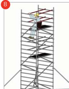
Using the 3T method. Clip 4 horizontal braces to the 19<sup>th</sup> and 21<sup>st</sup> rungs on both sides of the platform.
