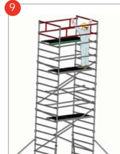
Fit two guardrail frames and lock. Fit two bracing frames and one plain platform on the opposite side. Then remove the horizontal brace from inside the platform and place on the lower rung.
