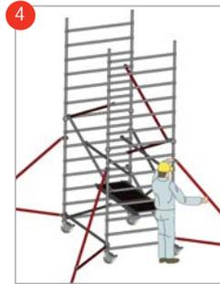
Continue diagonal bracing in a zig-zag pattern by attaching 2 diagonal braces on each side (5<sup>th</sup> to 8<sup>th</sup> and from the 8<sup>th</sup> to the 11<sup>th</sup> rungs). Fit stabilisers to the base unit - see separate section on stabilisers below.
