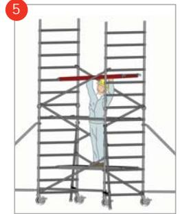
Fit trapdoor platform to the 10<sup>th</sup> rung of the tower.
