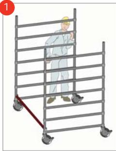
Insert castors and adjustable legs into the 7th rung frames. Clip horizontal brace onto the vertical member just above the 1<sup>st</sup> rung, with claw facing outwards.
